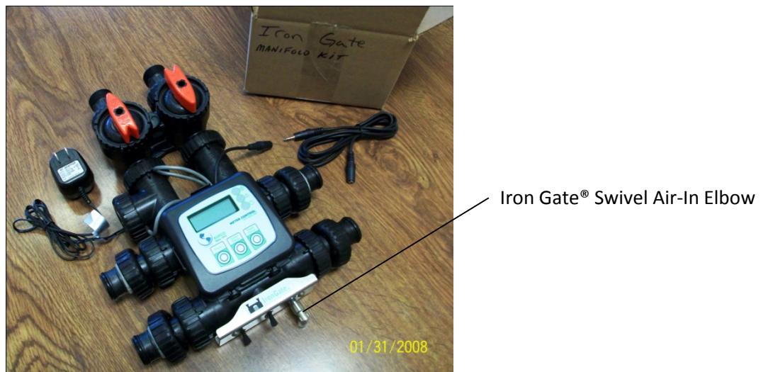
Figure 2 – Iron Gate Meter Control Assembly
