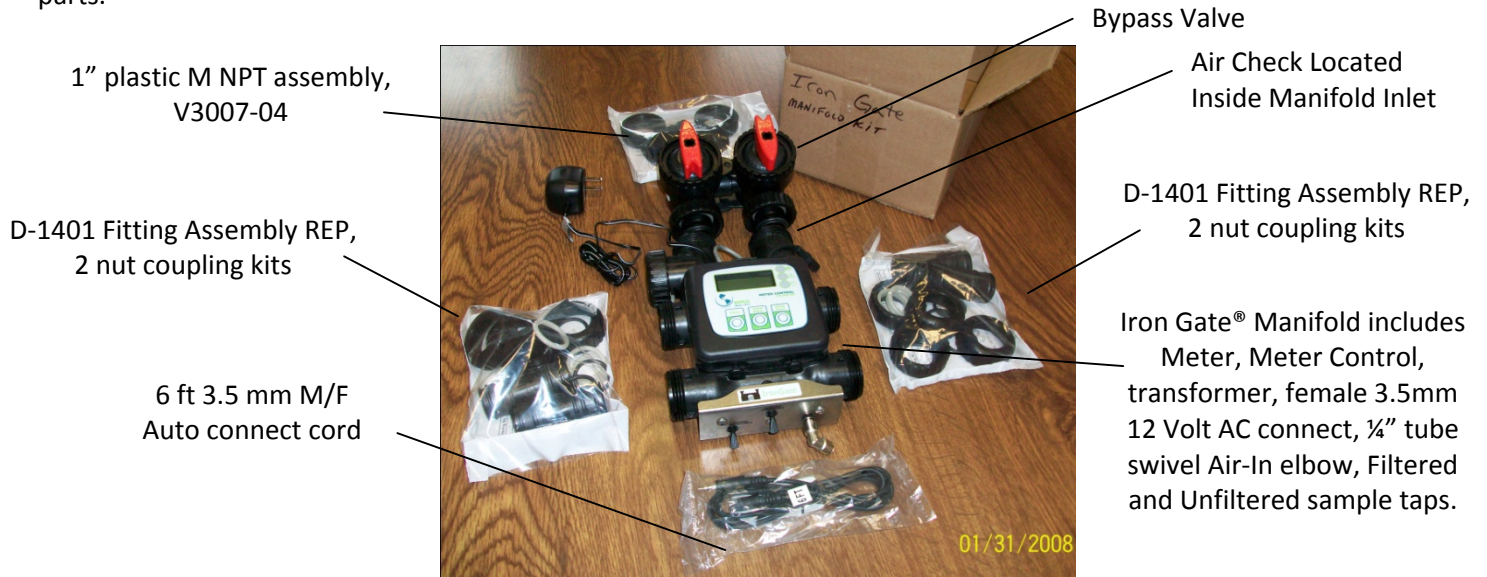
Figure 1 – Iron Gate Meter Control Parts
